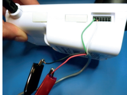
Figure 35 Auxiliary power supply connection
