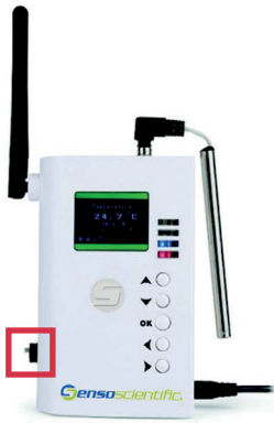
Figure 40 Vaccine refrigerator node with switch up
