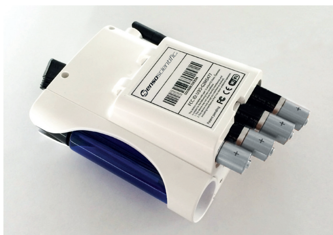
Figure 3. Insertion of batteries
