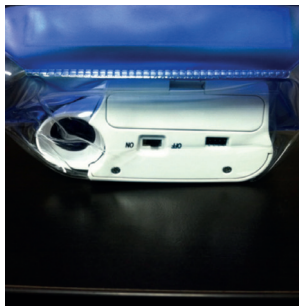
Figure 7 Note flat surface when pulled back, once it is properly fitted, zip the bag, fold the zip lock, and stick to velcro
