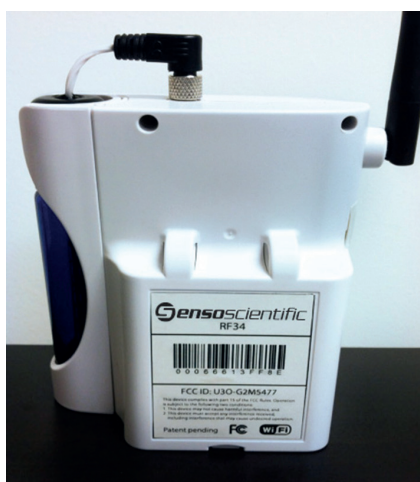
Figure 2. Barcode label with MAC address
