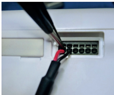
Figure 37 Inserting the wires
