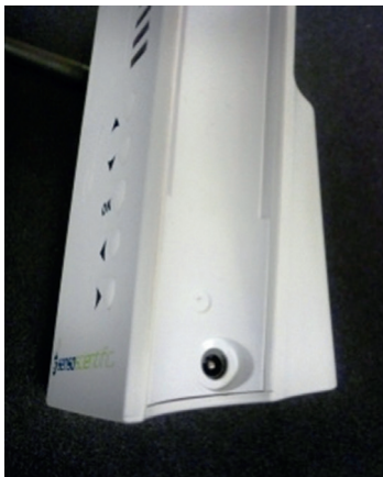
Figure 39 External power supply connector
