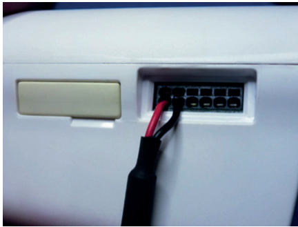
Figure 37 Inserting the wires
