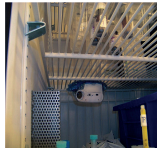
Figure 9 Mounting the node in a refrigerator
